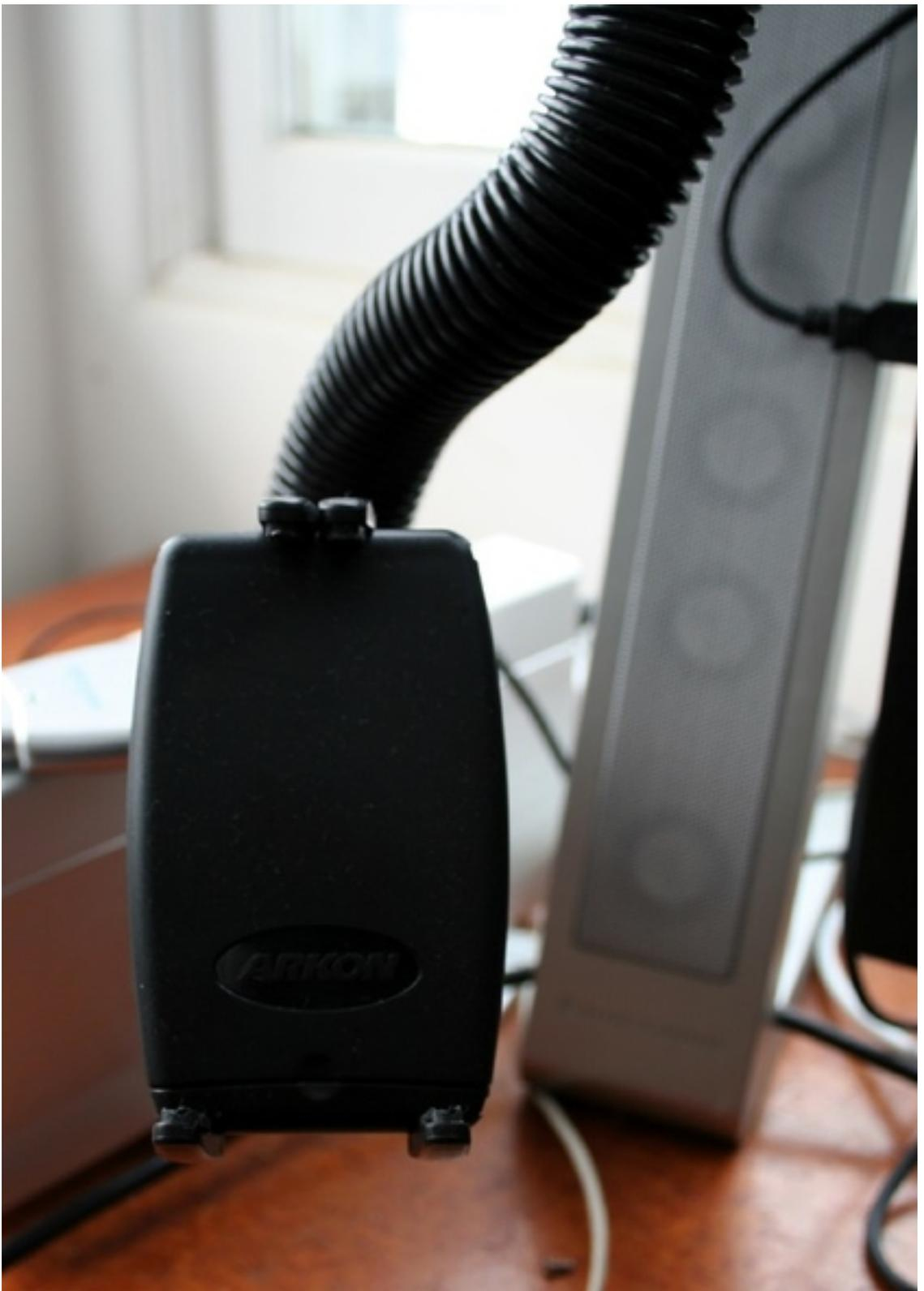
At the other end is a flat plate with four movable “fingers” on it. The bottom portion of the plate is on a spring-loaded slide, allowing the Raptor to hang onto any small electronic device up to about the height of an iPhone in a typical case (about 5”).
