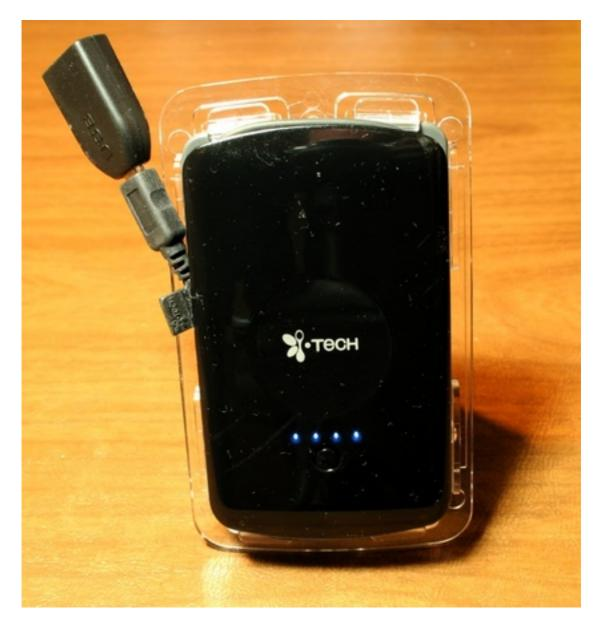
The button on the back can be pressed to show the state of charge of the internal battery. Here the SolarCharger has a full charge. A small red LED below the button illuminates steadily when charging via USB and flashes when charging from solar power.
