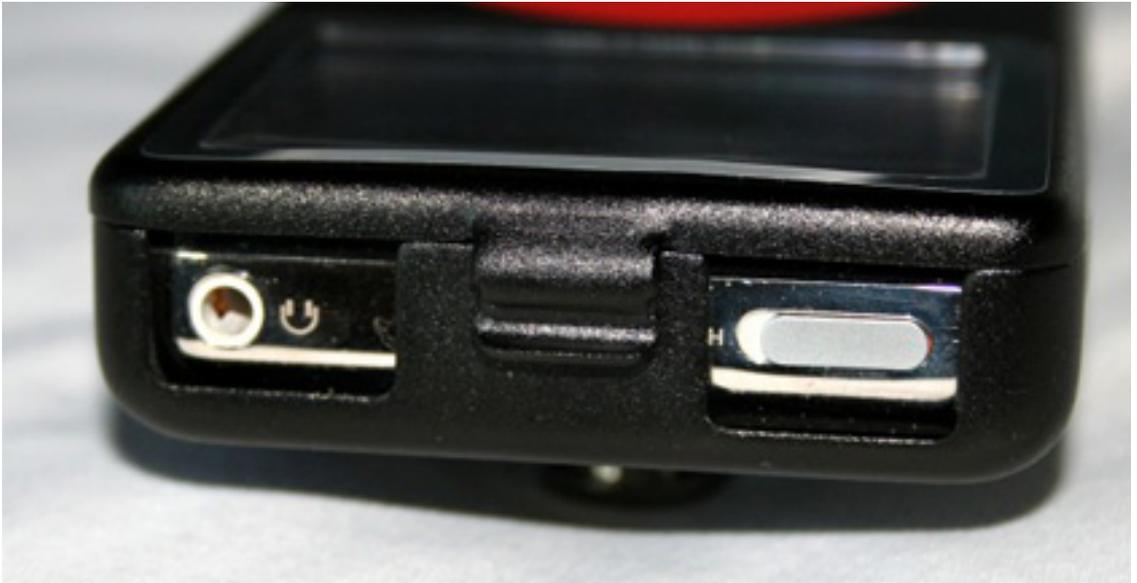
Shows access to hold switch and headphone jack, as well as clip holding the case together.
