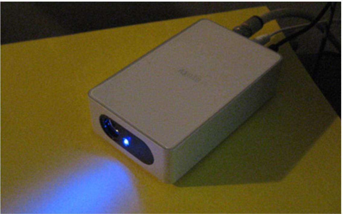
The EyeTV 250 hardware unit isn't just a converter box to let data flow through a coax cable into a Mac's USB port. The device also contains a compression chip which converts the incoming data into MPEG-1 or MPEG-2 format. Sure, my computer could do that, but it'd be highly processor-intensive. Since the EyeTV 250 is doing the heavy lifting, "older" computers (like my two-year-old PowerBook G4) can be used to watch and record TV.
